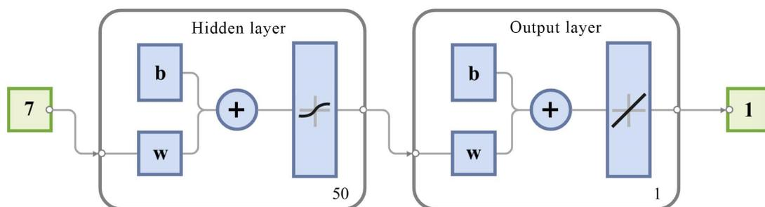
Fig. 2. Proposed topology of a neural network designed for learning from experimental data, **b** – bias, **w** – weights
