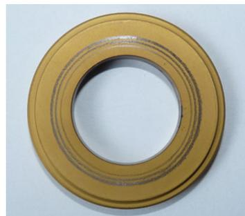
Fig. 1. Specimen with wear marks (TiN coating)
