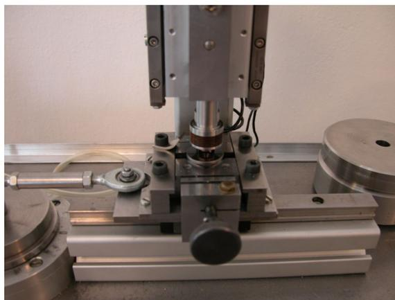
Fig. 2. Reciprocal tribometer developed at HVM Plasma Ltd
