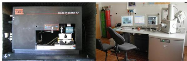
Fig. 3. Nanoindenter XP and SEM Quanta 200
