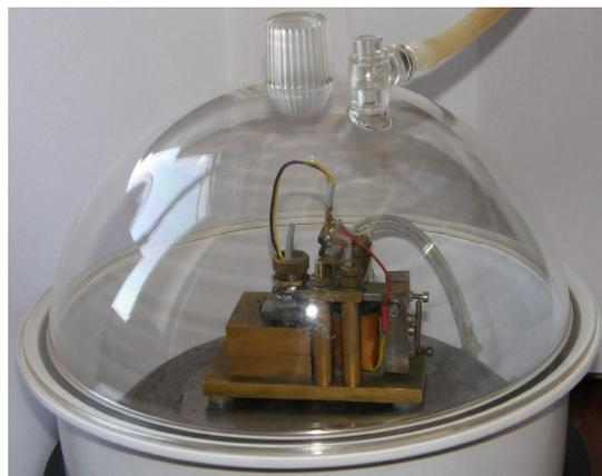
Fig. 1. Impact tester developed at the Institute of Scientific Instruments ASCR, Brno for measurement in controlled environment
