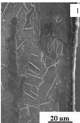
Obr. 2. Hrubé ihlice \text{Fe}_4\text{N} nitridov
