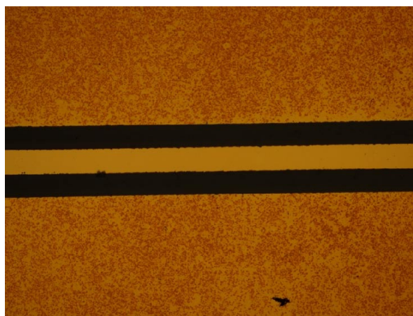
Fig. 1. Detail of the deposited layer of the gold nanoparticles (wide strips) and uncovered counterelectrode ( \sim 100 \mu\text{m} narrow strip)
