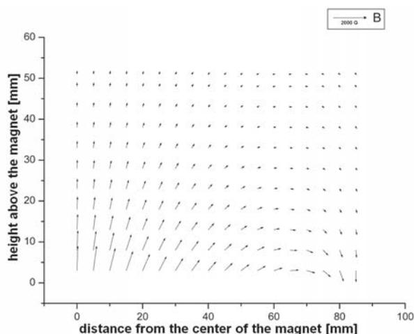
Fig. 2. Sketch of the magnetic field configuration
